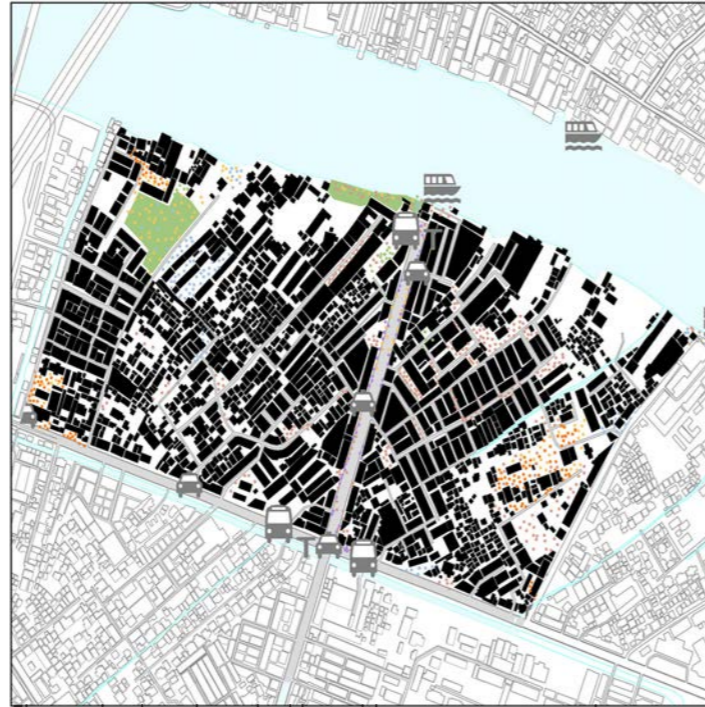
Fine-grain, densely packed but with open spaces near river Single arterial road imposed onto diagonal grid 5 primary public transportation modes (Bus, Rail, Taxi, Boat, Tuk-tuk.) ~10 transportation nodes
